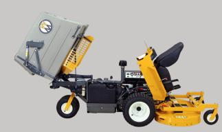
Tilt-Open bodies quickly expose engine and drive train for service and easy maintenance.
