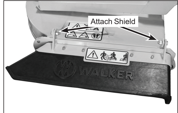
Discharge Shield Installation on Side Discharge Deck
