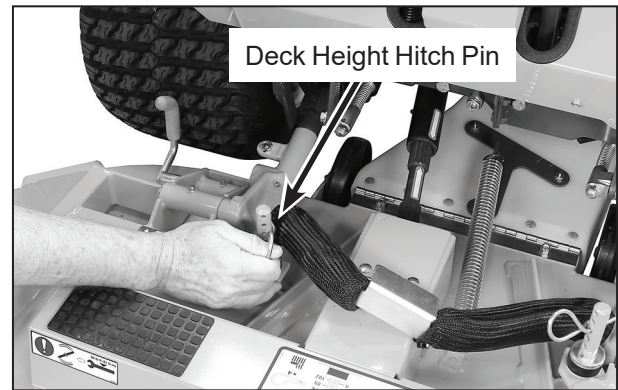
Remove One Deck Height Hitch Pin
