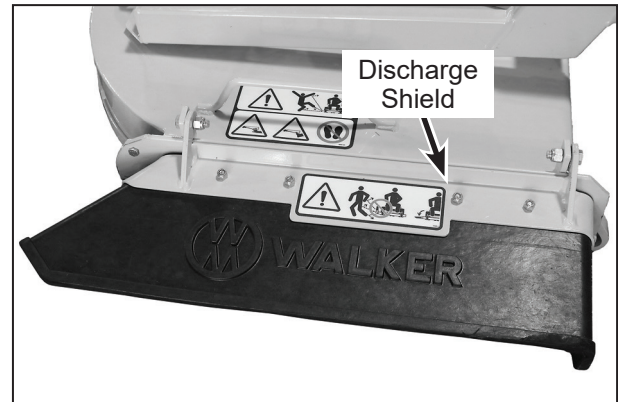
Side Discharge Deflector Shield in Lowest Position
