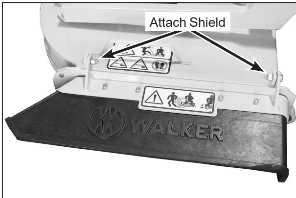
Discharge Shield Installation on Side Discharge Deck
