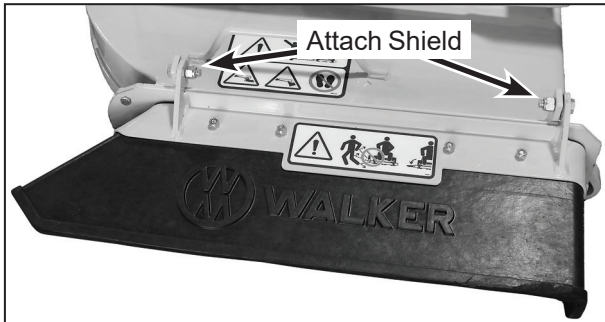
Discharge Shield Installation on Side Discharge Deck
