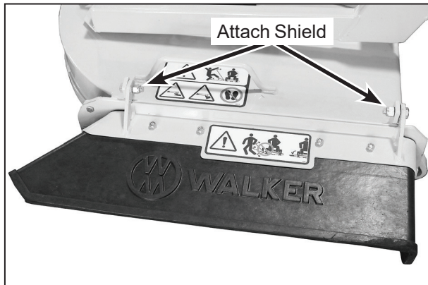
Deck Discharge Shield Installation
