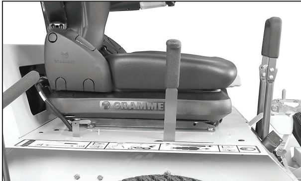
Correct FSC Lever NEUTRAL-PARK Position
