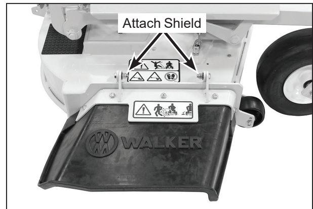
Deck Discharge Shield Installation
